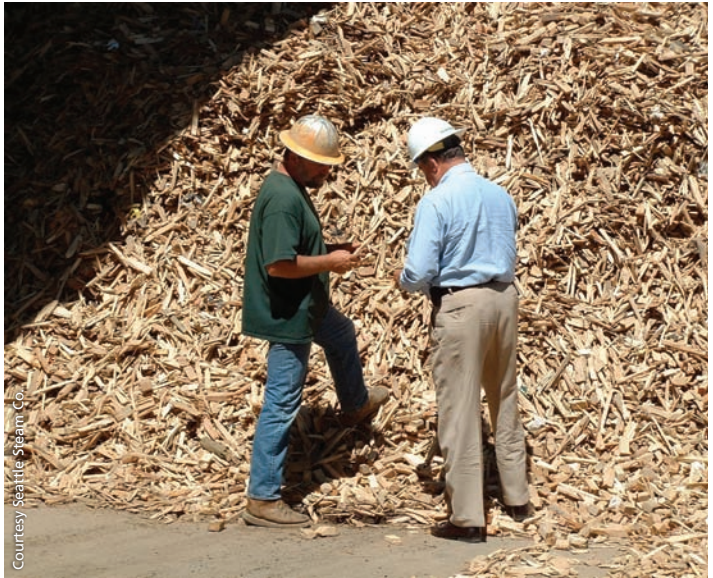
Seattle Steam uses urban waste wood as the fuel source for its new boiler. The wood comes in all shapes and sizes (left) before it is processed to meet the company's boiler specifications (right).
