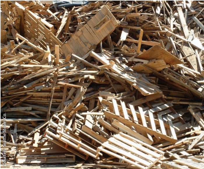
Seattle Steam uses urban waste wood as the fuel source for its new boiler. The wood comes in all shapes and sizes (left) before it is processed to meet the company's boiler specifications (right).
